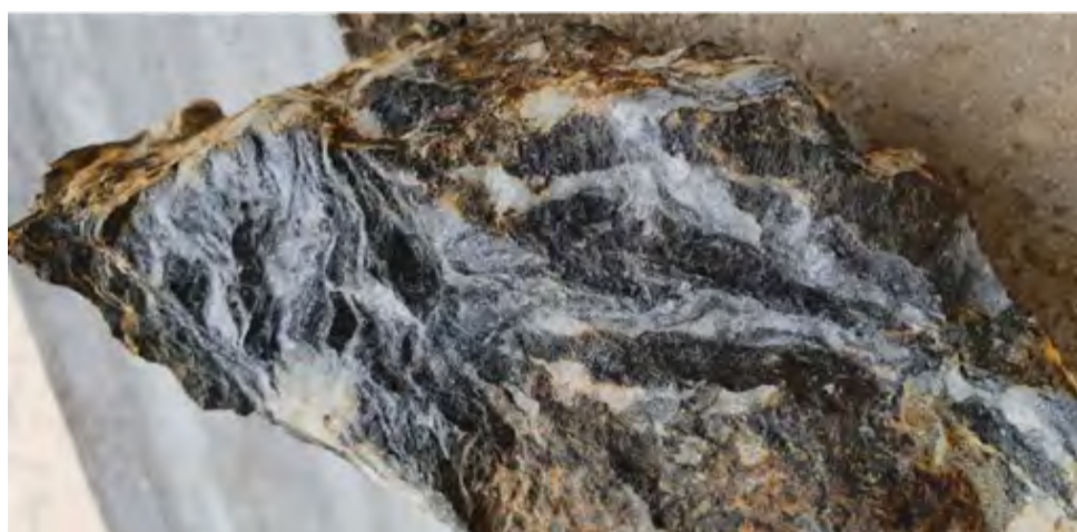
Kampion shkëmbor me mineralizime polimetalore si më poshtë [Rock sample with polymetallic mineralizations as follows] SiO 2 -87.8%, Al 2 O 3 -2.9%, Fe 2 O 3 -0.99%, CaO-1.68%, MgO- 1.31%, MnO - 0.01%, NiO - 0.009%, CuO - 0.55%.
